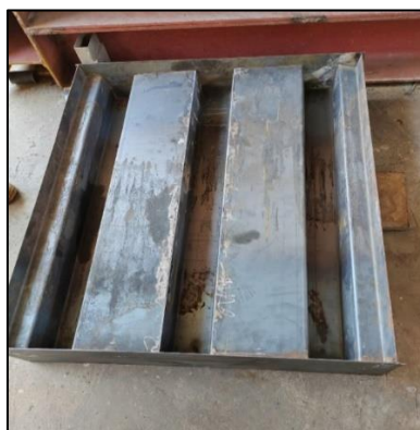
Plate (1): Steel mold formworks
