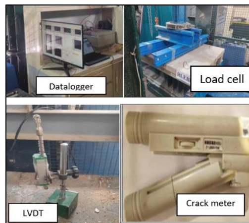
Plate (5): the instrumentations used in the test of the specimens
