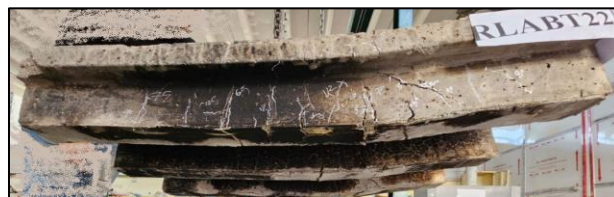
Plate 7: Cracking patterns for all tested slab specimens
