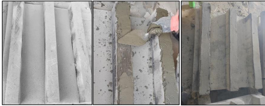
a. scratching the surface b. mortar layer applied over the mesh c. specimens after cured
