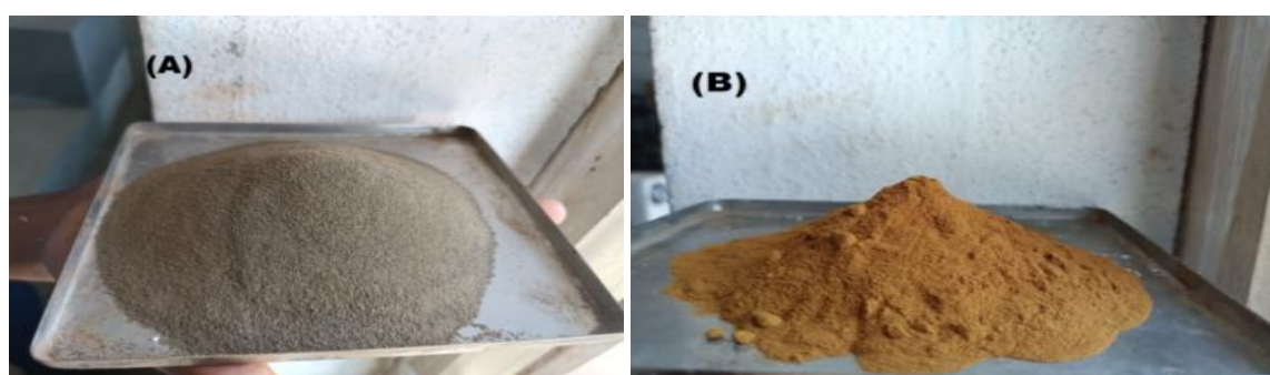
Figure 1: (A) Black cotton soil (B) Calcium lignosulfonate
