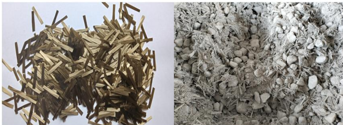
Figure 1. Chopped Basalt Fibres (Left) and Their Uniform Distribution in Dry Concrete Mix (Right) Concrete was proportioned to achieve a characteristic compressive strength of 40 MPa at 28 days using guidelines from IS: 10262–2019. The mix incorporated fly ash as a partial cement replacement to improve durability. The final proportions are presented in Table 2.
