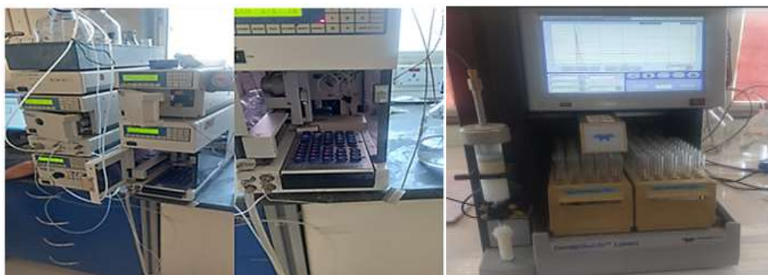
Fig.3. Instrumentation used for phytochemical analysis: (A) JASCO HPLC Autosampler for quantification of gallic acid; (B) Combi Flash RF+ Lumen system for purification of bioactive compounds.
