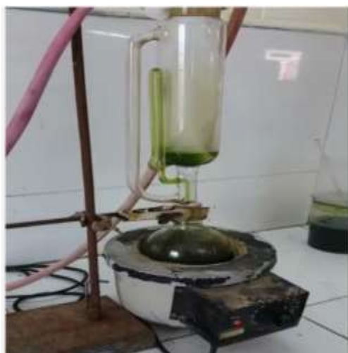
Figure 3.2: Soxhlet Apparatus Used for Extraction of Epipremnum aureum
